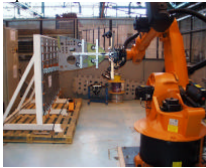
Figure 8. The Kuka robot and assembly end-effector
