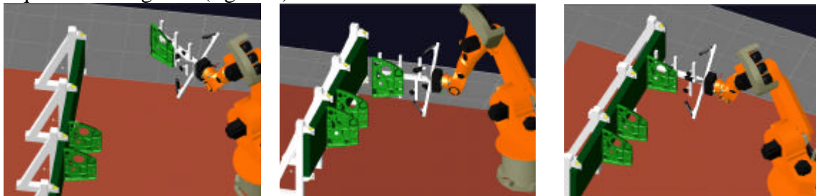
Figure 1. The robot picks up a component (e.g. track rib) and delivers it to approximately the correct location where it is then guided into position by the measurement system
