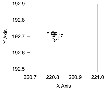
Figure 5. Target image location positions for a stationary target
