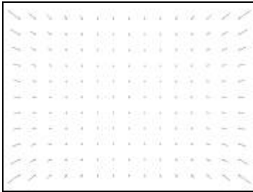
Figure 1. Radial lens distortion vectors
