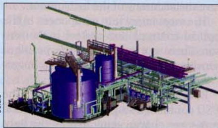
The Proscan scanner (left) measures surface finish. Soisc's system produces CAD data (above) from multiple scans of a scene (right).
