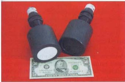
Figure 8. (Above) Example ultrasound system - Aigatron Range: 1.8 meters; Stand off 200 mm. Resolution: 1.7 mm Measurement frequency: 28 Hz
