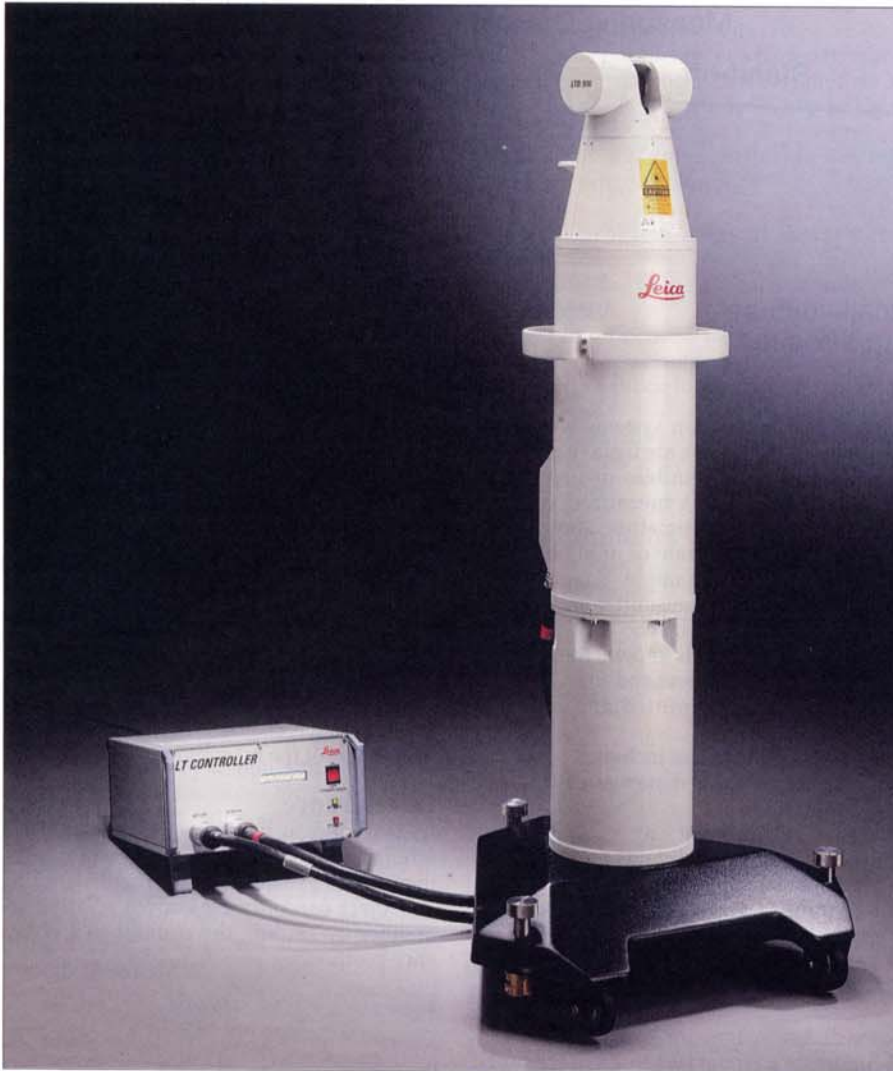
Figure 12. Example of a laser tracker system Leica Laser tracker LTD 500 Range: 70 metres. Stand off: 150 mm. Resolution: (angle, distance + 5 ppm) (0.07", 1.26 µm + 5 µm / metre) Measurement frequency: 1000 Hz
