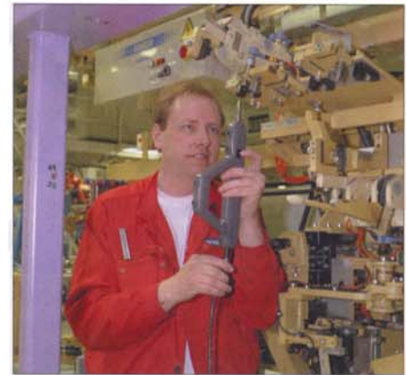
Figure 6. Photogrammetry example system Metronor portable CMM Range: 2 metres. Stand off: 8 metres. Resolution: 0.01mm. Measurement frequency: 1 Hz
