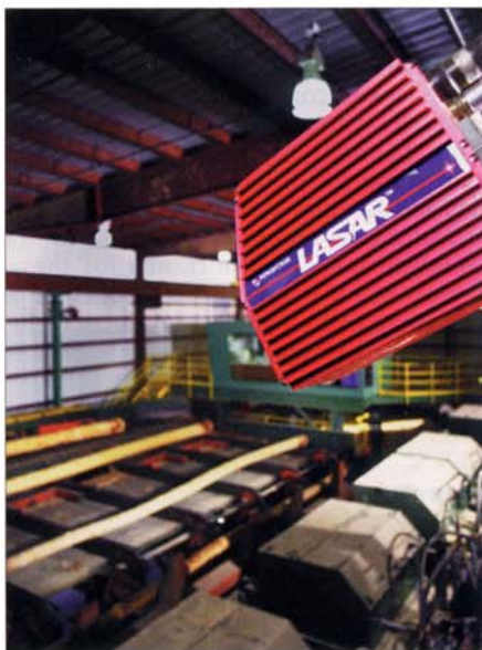
Range: 38.5 metres Stand off: 1.5 metres Resolution: 2-500 mm depending on range Measurement frequency: 190 scanned lines per second
