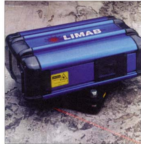
Figure 2. An example of a triangulation instrument: Limab LMS 6035S. Sensor range: 2000 mm Stand off: 300 mm Resolution: 0.1 mm Measurement frequency: 500 Hz max
