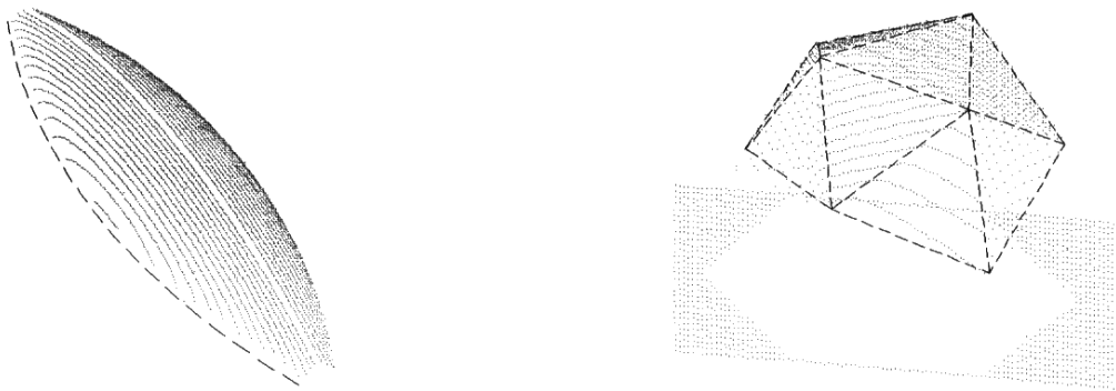
Fig 2. Cross sections of a model boat hull and polyhedron obtained by optical triangulation.
